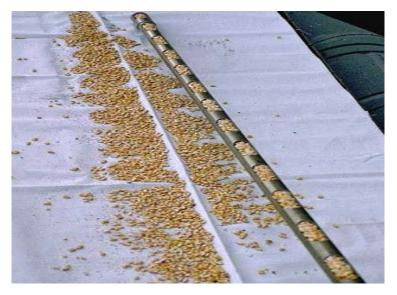
Fig: (2) Probe after collection of increment sample
